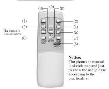
The **cooling only units** don't have the function of heating or electric heating. When the remote controller turns to such function buttons, the units will not result such effect.
